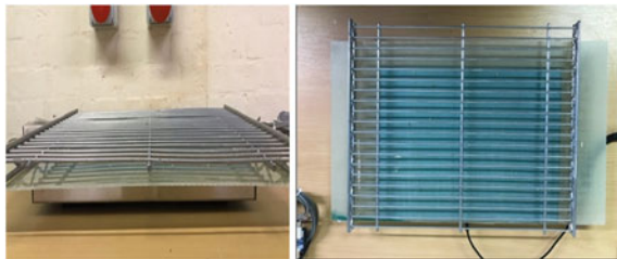
Fig. 2 Experimental setup. (1-infrared camera on a tripod, 2-digital scale, 3-drying rack, 4-heater hood, 5-Lid (green body), 6-K type thermocouples, 7-temperature data logger (TC-08), 8-Humidity Datalogger (Dr Daq), 9-Dr Daq humidity sensor)
