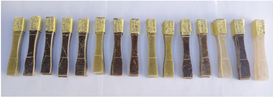
Fig. 1 Tensile test samples of post-consumer glass and sawdust reinforced polyester composites
