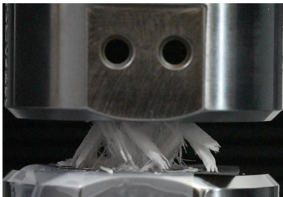
Fig. 5 Photograph of the collapsing process during compressive test of alumina scaffolds with 10vol% solid content
