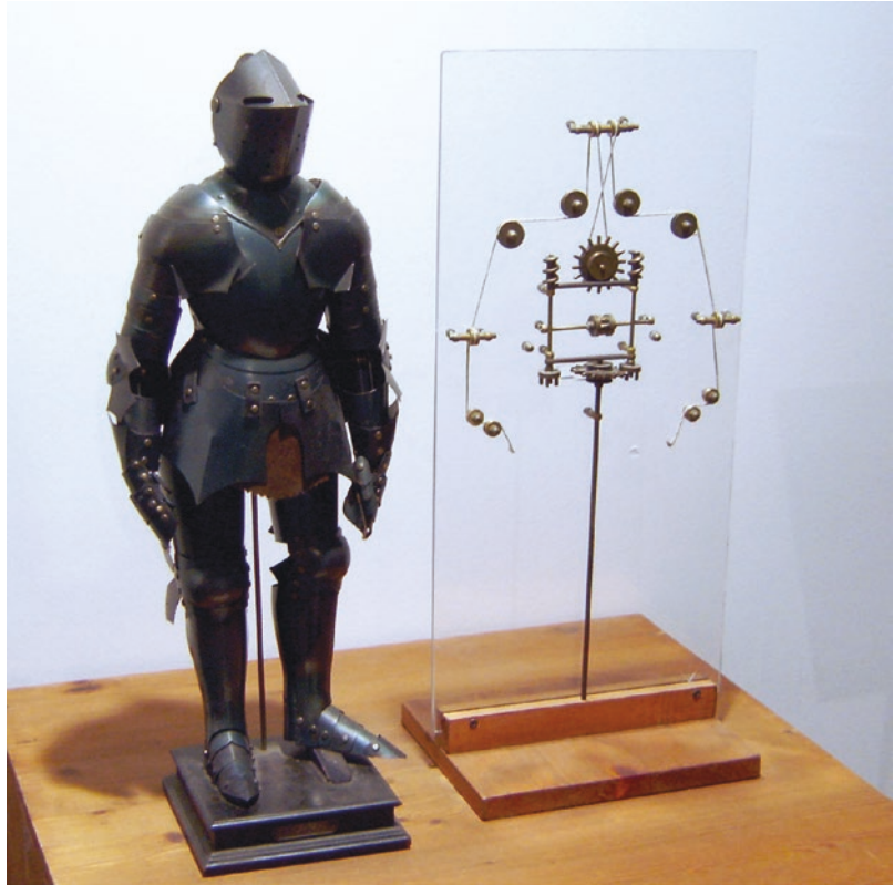
Fig. 26.1 The “Metal-Plated Warrior” designed by Leonardo da Vinci in 1495, the first robot that imitated human movements of the jaw, arms, and neck
