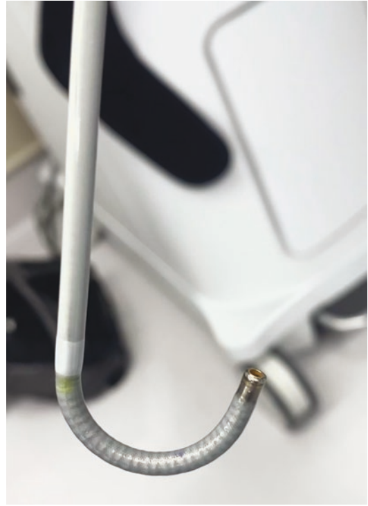
Fig. 26.9 The shape-sensing catheter of the Ion platform
