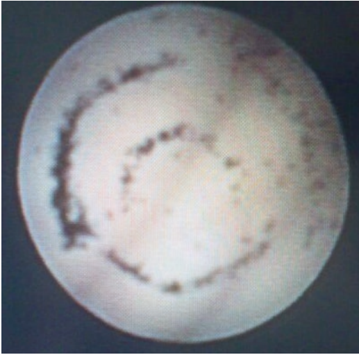
Fig. 3.3 Black dots corresponding to broken fibers after the ultrathin fiberoptic bronchoscope was accidentally bitten by a patient
