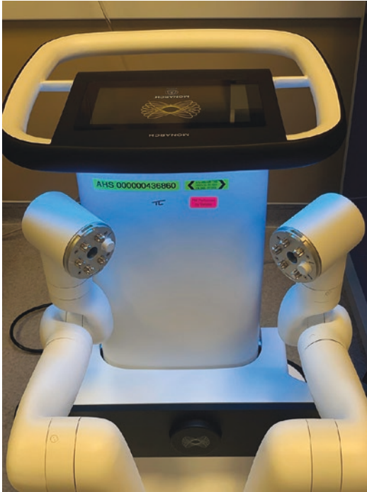
Fig. 26.4 The robotic arms of the Monarch platform
