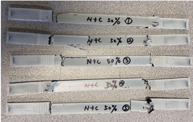
Fig. 9 The failures of Nylon-42.3%CF tensile test samples (50% represents half carbon fiber layers and half nylon layers, and for this type of test samples, the carbon fiber volume fraction is 42.3%)
