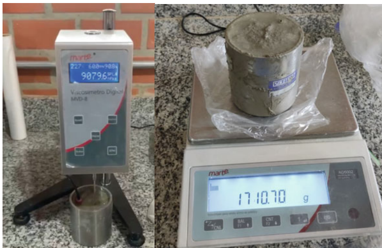
Fig. 3 The viscosity measurement (left) and density testing device (right)
