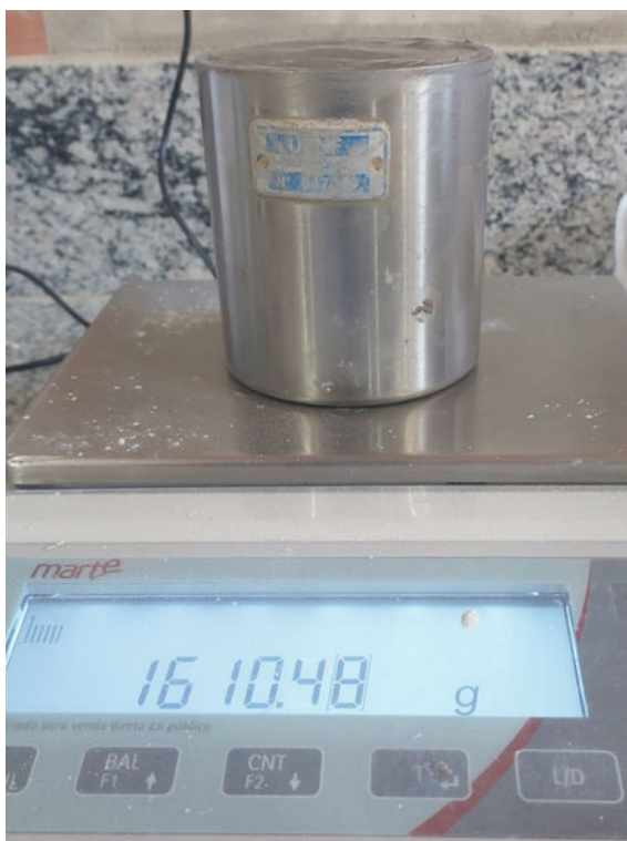
Fig. 2 Dough density test in the fresh state
