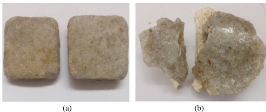
Fig. 1 a Glass ceramics obtained from cooling at 1 °C/minute. b Glass ceramics obtained from cooling at 5 °C/minute
