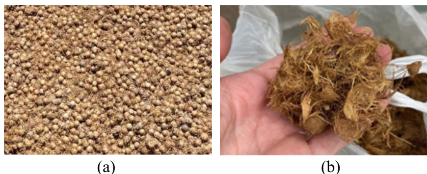
Fig. 1 Açai waste: a seeds with fibers; b fibers
