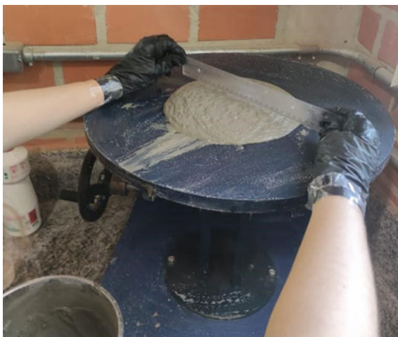
Fig. 2 Reference paste consistency test - Flow table
