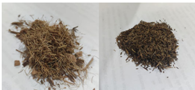
Fig. 1 On the left the coconut fiber and on the right the fibers of the pineapple crown leaf (PALF)
