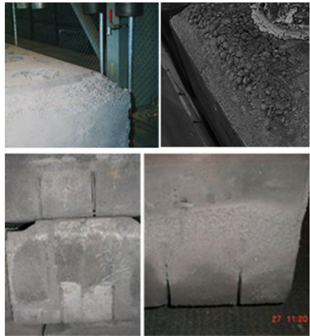
Fig. 1 Examples of free dust on anodes. The cause of all of these defects is known, as are the solutions. Unfortunately, it is still common to see anodes set in cells with these problems. From [2]
