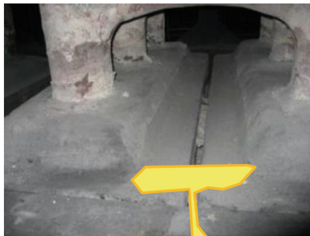
Fig. 5 Anode top profile recommended by Barry showing how a surge reservoir for bath overflow is formed; this reduces stub flux wash. From [2]
