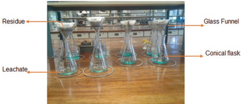
Fig. 5.4 Gravity-driven filtration process of copper recovery from WCD
