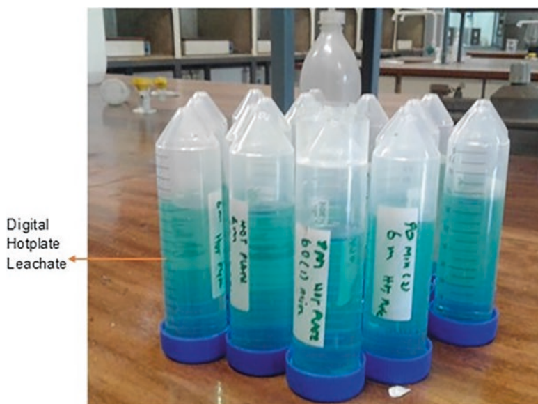
Fig. 5.9 Leachate from hotplate leaching
