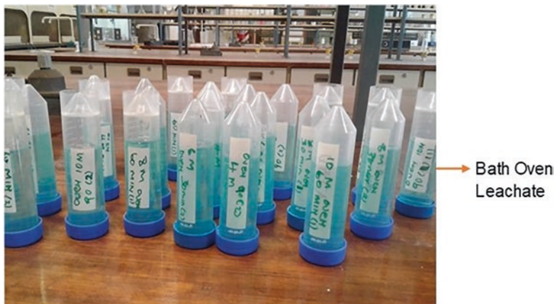
Fig. 5.10 Leachate from oven leaching
