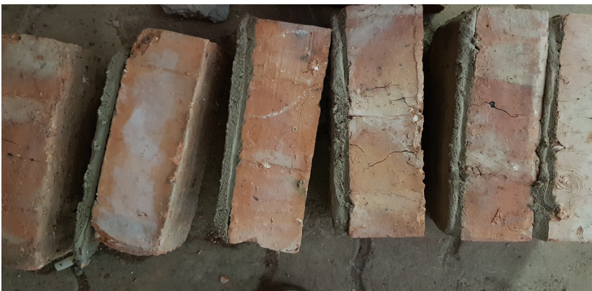
Fig. 5. Dry laid burnt clay brick prism failure mode.
