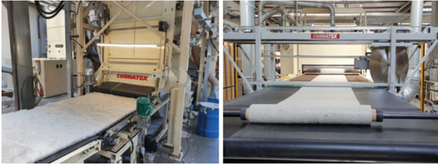
Fig. 17 Cormatex industrial production of rGF mat
