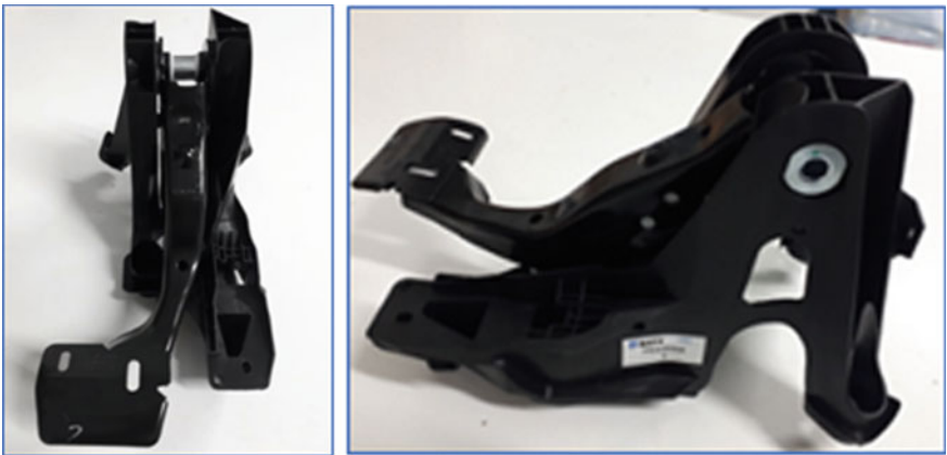
Fig. 7 Pedal bracket prototype ready for validation test
