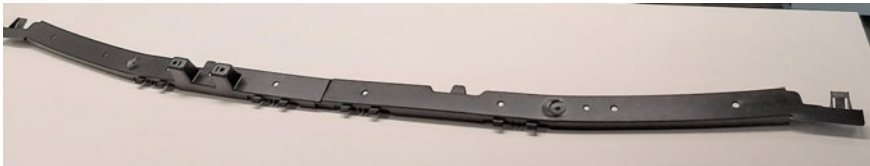
Fig. 16 Prototype cowl top support with rGF
