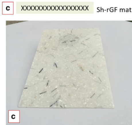
Fig. 23 Sample made with Sh-rGF mat
