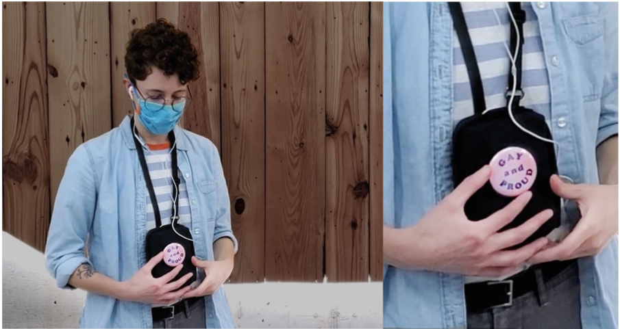
Fig. 6. A second view of the Button Portraits interaction: A participant chooses a button to wear on their audio player, places it on a magnetized area, and listens to an oral history story fragment corresponding to that button. Each button has a unique NFC tag read by the audio player.
