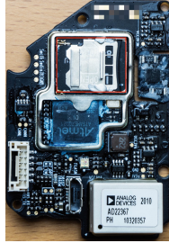
Fig. 1. Flight recorder module of the DJI Inspire 2 with a glued-in microSD card (top, marked in red). (Color figure online)
