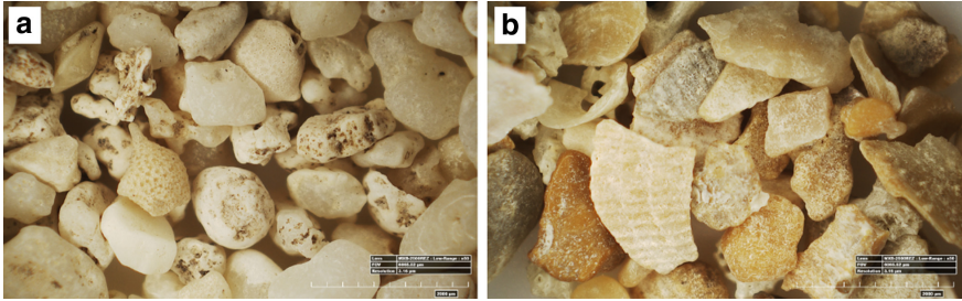
Fig. 2. Macroscopic photograph of the two sands a Classica marine aragonite b Barry's beach sand. The photographs were taken on sieved samples. Hence, the grain sizes are between 0.6 and 1.18 mm
