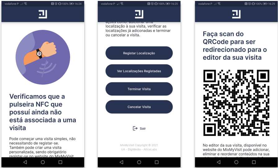
Fig. 5. Sample screens of the mobile application (left: initial screen after scanning NFC tag not associated with any visit, in the middle: the main menu of the visit, right: QR-code presented to redirect the user to an online video editor).
