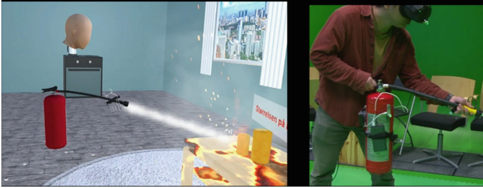
Fig. 1. Holding the “real” nozzle, and press the “real” handle to spray “virtual” foam to extinguish “virtual” fire
