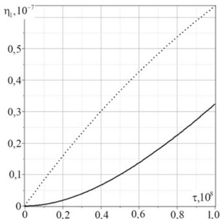
**Fig. 9.8** Zinc concentration increment  $\eta_1(x_1, x_2, \tau)$ . The solid line corresponds to the time  $\tau^{(q)} = 200$  s, the dotted line to  $\tau^{(q)} = 0$
