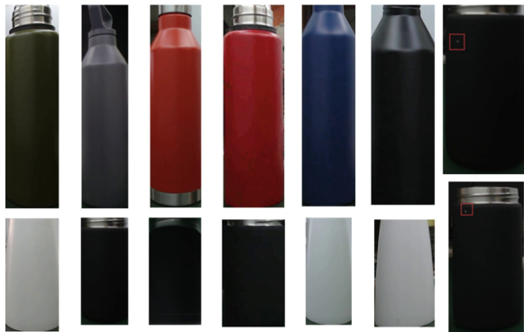
Fig. 2. Samples of the ZeroBox bottle product dataset. Defective parts are labeled in the red squares. (Color figure online)
