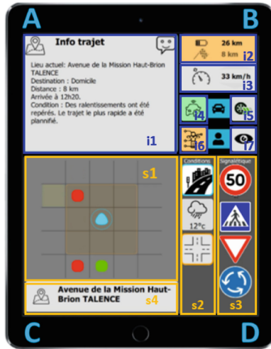
Fig. 3. Correspondence of the interface fields: i1 = contextual information; i2 = autonomy and remaining distance; i3 = speed, acceleration and deceleration; i4 = technical status of the AV; i5 = dynamics; i6 = passenger status detection capability; i7 = passenger status; s1 = radar; s2 = conditions; s3 = signaling; s4 = location. (Color figure online)
