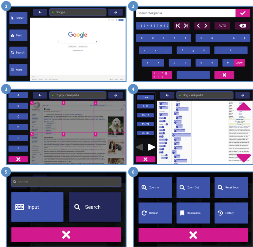
Fig. 5. Screenshots from Boggle’s interface showing the (1) home menu with basic navigation and reading controls, (2) an 18-target keyboard interface with auto-completion facilities, (3) on-page region selection control (to activate links/buttons/text fields in a particular region), (4) on-page link/button/text field selection control (numbered), (5) in-built Google search menu, as well as (6) page and bookmark management facilities.
