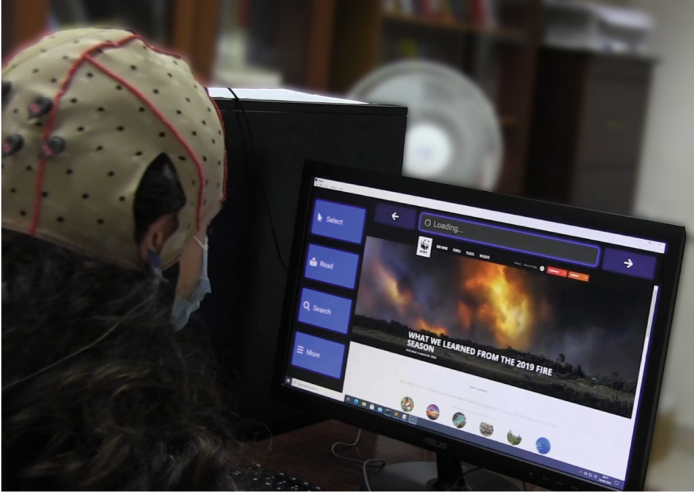
Fig. 3. User interacting with Boggle via asynchronous, BCI-based control.
