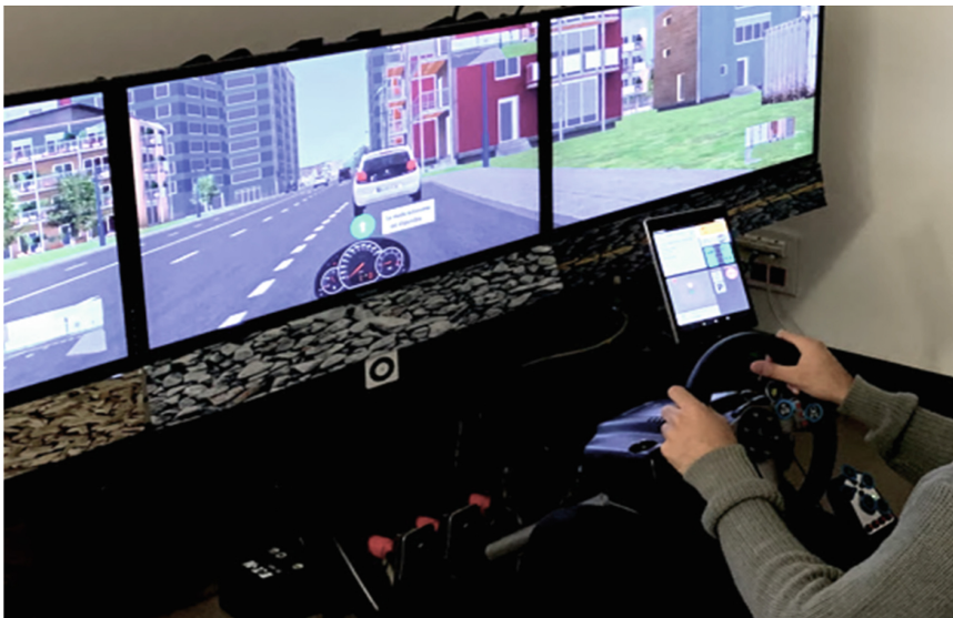
Fig. 4. Visual of the HMI implementation on the ScannerStudio 1.9 simulator. The image (taken from a video) allows to see on the radar the presence of a pedestrian (yellow square) and a distant car on the right lane (green circle). (Color figure online)
