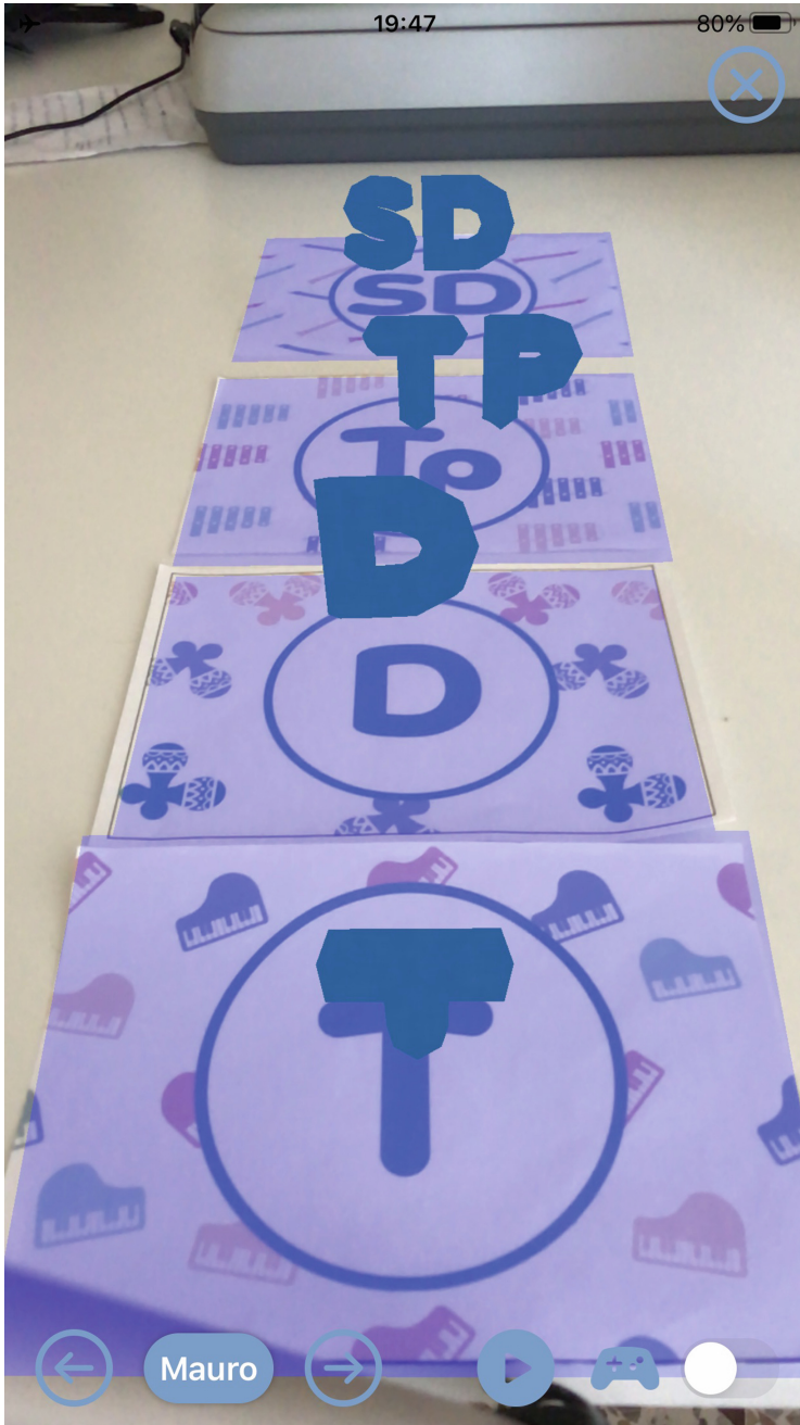
Fig. 10. Recognition of markers and superimposition of chord symbols in AR. Image taken from [3].
