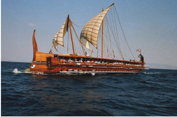
Fig. 3.1 An HS Olympias trireme replica. It was built in 1987, funded by the Hellenic Navy, and is now purely on exhibit. During the original sea trials, each oarsman required at least 1 L of water per hour or 8 L per person during a full day of rowing [5]. (Source: Hellenic Navy. Available at: https://www.hellenicnavy.gr/en/history-tradition/ships-museum-exhibits/trireme-olympias.html )
