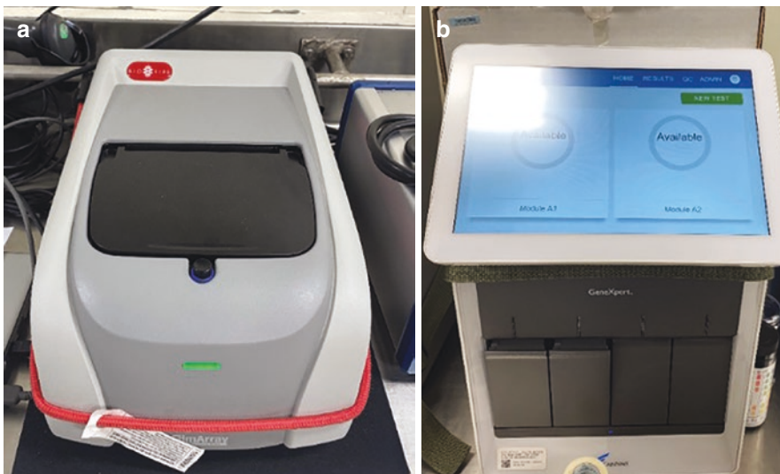
Fig. 8.4 Systems for detection of common viral pathogens, only found on larger deployed maritime platforms (a) Biofire FilmArray (b) Cepheid GeneXpert. (Source: Photos courtesy of Clara A. Pangco, MLS)
