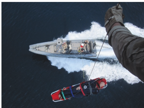
Fig. 31.9 11-Meter Rigid Hull Inflatable Boat (RHIB) patient hoist simulation. (Source: Photo courtesy of Wayne Papalski, Search and Rescue Medical Technician)
