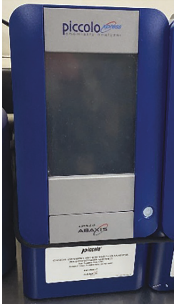
Fig. 8.3 Sample chemistry analyzer for deployed platforms: the Piccolo Xpress. (Source: Photo courtesy of Clara A. Pangco, MLS)
