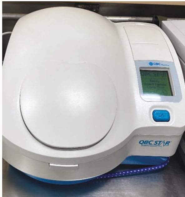
Fig. 8.2 Standard hematology system on deployed platforms: the QBC Star. (Source: Photo courtesy of Clara A. Pangco, MLS)
