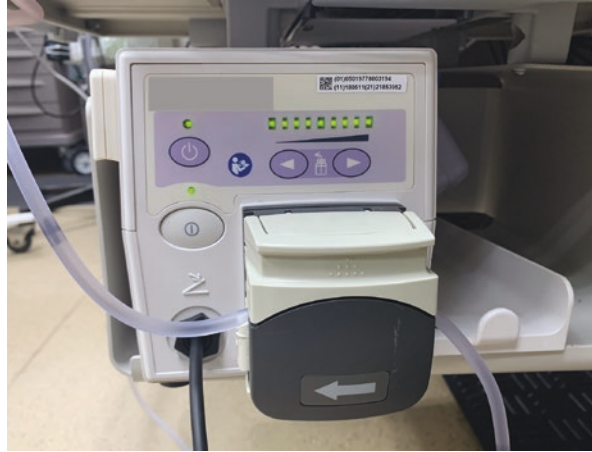
Fig. 18.4 Water irrigation pump with arrow indicating direction of water flow. (Source: Photo courtesy of R. Daniel Lawson, MD)
