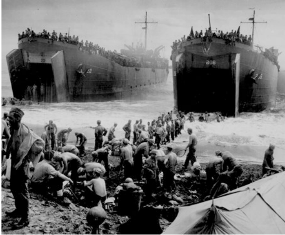
Fig. 3.8 Landing Ship, Tank (LST) unloading cargo onto the beach. They were built during World War II to support amphibious operations—able to land vehicles, cargo, and troops directly onto the shore. During the amphibious assault at Iwo Jima in 1945, four LSTs were augmented with surgical teams. (Source: Government publication, not in copyright. Available at: https://www.archives.gov/files/research/military/ww2/photos/images/ww2-151.jpg )
