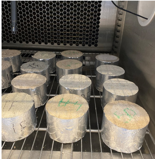
Fig. 4. Hemp concrete samples in a climatic chamber for MBV measurements
