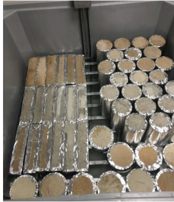
Fig. 2. Accelerated aging setup (Partial immersion)
