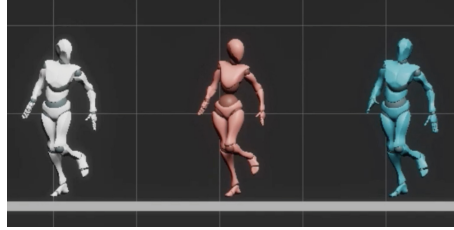
Fig. 7. Avatar comparison when placed alongside. Red avatar is the source, blue is the estimated pose and white is the sensor fusion (Color figure online)
