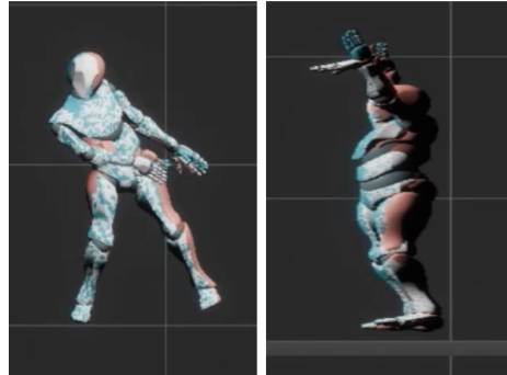
Fig. 8. Avatar comparison on overlapping. Red avatar is the source, blue is the estimated pose and white is the sensor fusion (Color figure online)
