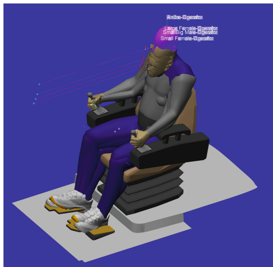
Fig. 12. Nominal position of the joysticks
