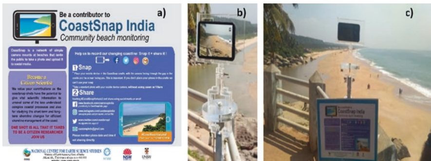
Fig. 26.4 CoastSnap. (a) Notice board with instructions. (b) Closeup view of the CoastSnap cradle. (c) CoastSnap Station at Adimalathura
