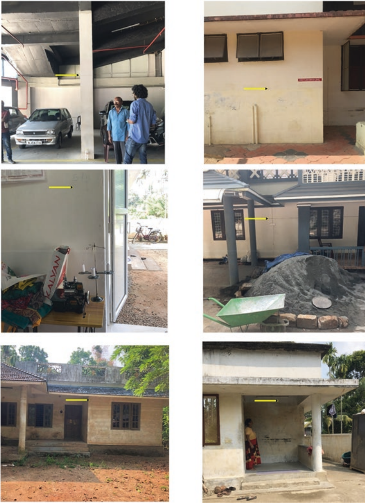
Fig. 5.2 Field photographs show flood levels in the study area
