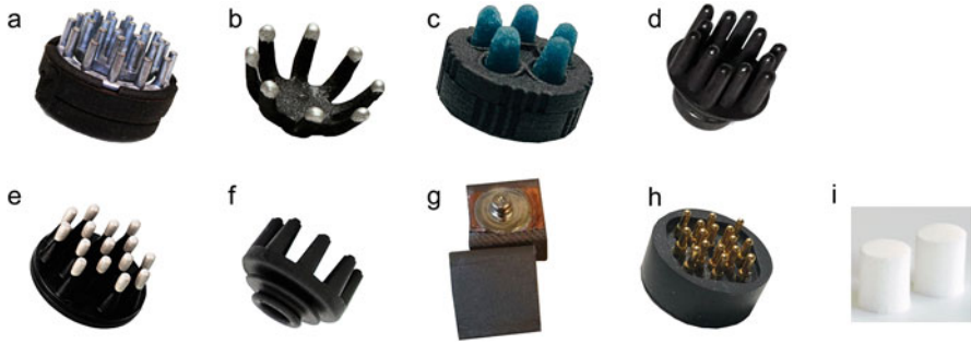
Fig. 7.7 Sensor types – several types of dry electrodes in the market. (a) Wearable sensing. (b, c) Cognionics. (d) OpenBCI sensor. (e) IMEC. (f) g.tec g.SAHARA. (g, h) MINDO. (i) mBrainTrain sponge sensor (semi-dry)
