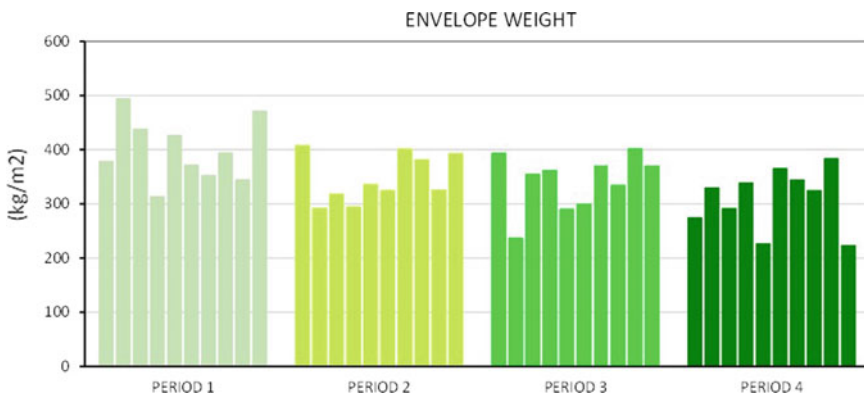
Fig. 9 Weight of the envelope component of the 10 dwellings analysed in each period
