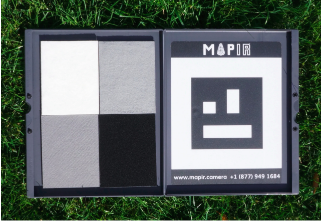
Fig. 9. MAPIR camera reflectance calibration ground target board.
