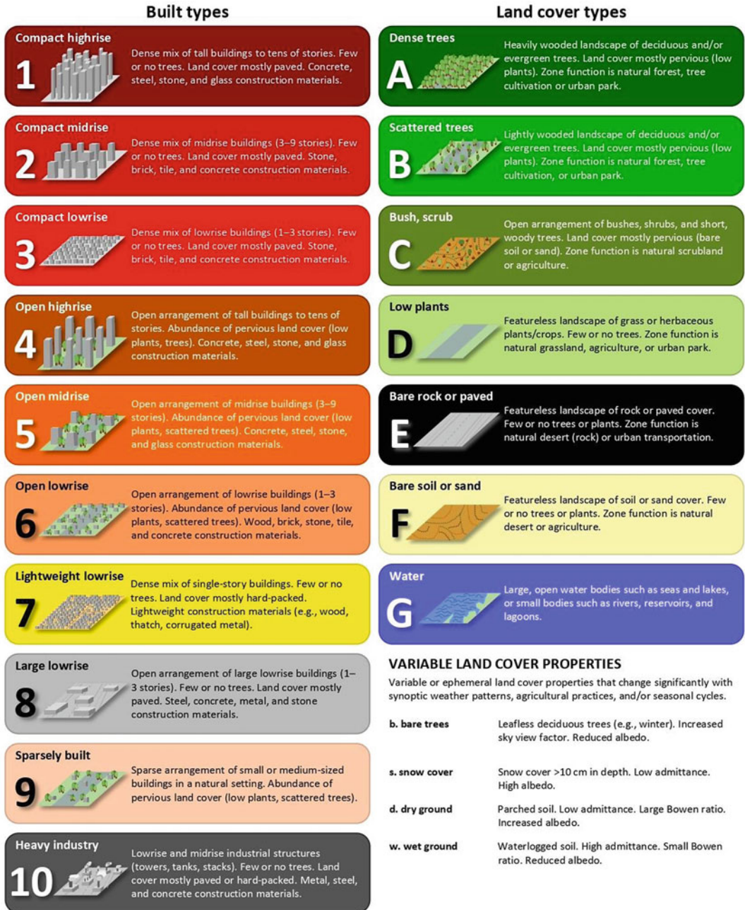
Fig. 16.5 Local climate zone typology. Source The World Urban Database and Access Portal Tools
