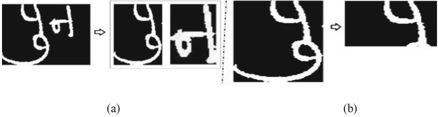
Fig. 6. (a) Illustration of connected component labeling (b) segmentation of lower modifier
