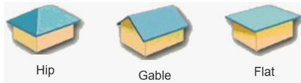
Fig. 5. Three most common roof shapes [2]
