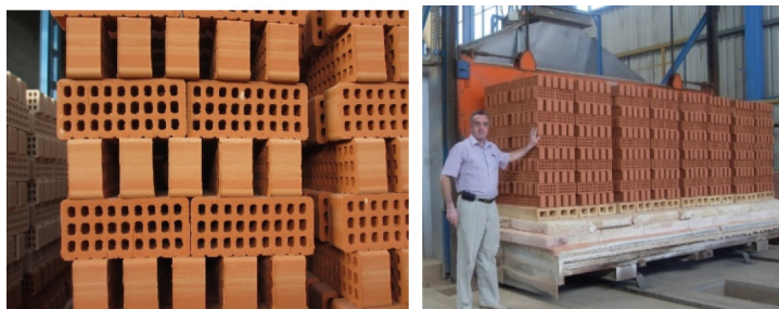
Fig. 5. Ceramic brick produced by compression method moulds based on clay types of supports
