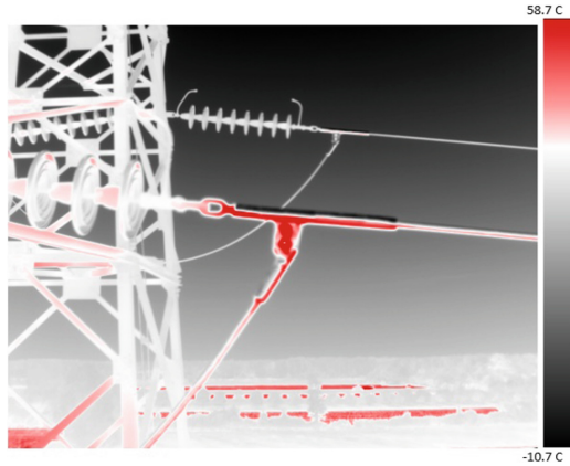
Fig. 8. Thermal image of a 110 kV transmission line made by an unmanned aerial vehicle with a 640 \times 512 camera and a 40.6^\circ lens
