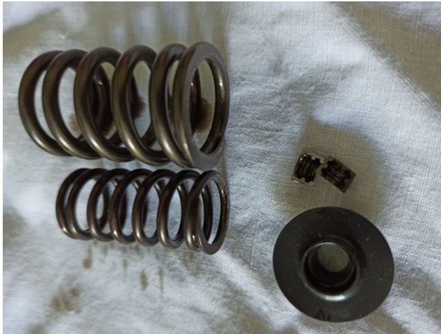
Fig. 16. Dismantled springs, round valve spring retainer plate and vale collet halves.
