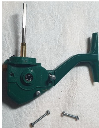
Fig. 15. Housing connection with the rod handle.
