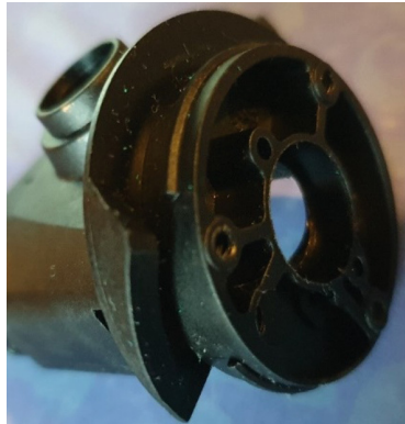
Fig. 2. The rotor cam wear.
