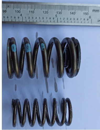
Fig. 3. Valve springs, outer (main), and inner (safety).
