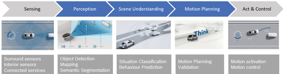
Fig. 1. Standard components of an AD system, modified from [57].
