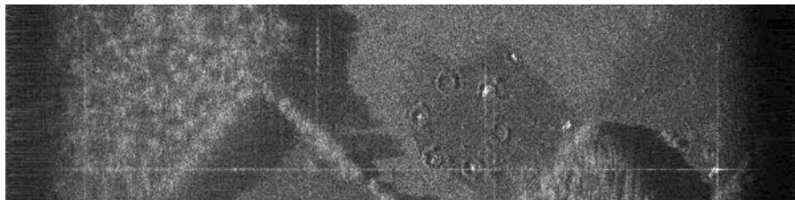
Fig. 2 A SAR image from Mission 78, Pass 1 collected by the Advanced Detection Technology Sensor (ADTS), an airborne SAR/RAR millimeter-wave sensor operated by MIT Lincoln Laboratory. The ADTS operates at Ka band (32.6 to 37 GHz) and was used to collect clutter and armor scenes using its stripmap mode
