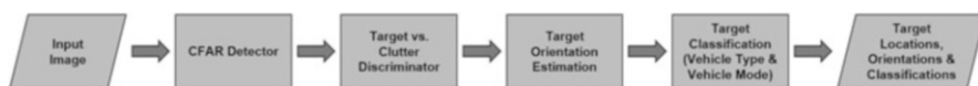
Fig. 4 The end-to-end SAR ATR processing chain. This section describes algorithms for the operations outlined in red
