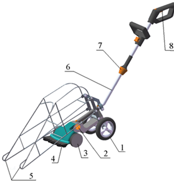
Fig. 2. Trimmer for breeding TS-0.2: 1 – wheel drive; 2 – cutterbar tilt adjuster; 3 – support roller; 4 – cutterbar; 5 – stem lifter - divider; 6 – handle; 7 - handle length adjuster; 8 – cutterbar on/off button.
