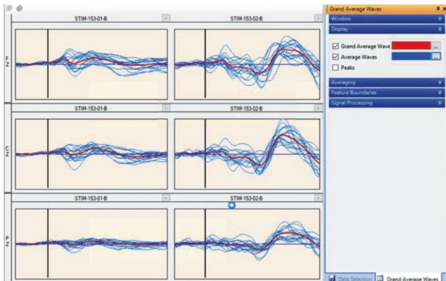
Fig. 17.4 In response to the deviant (oddball) tone during the auditory ERP paradigm, a large positive wave is produced over the 250–450 ms range with a peak around 300–350 ms range (P300). This P300 response is not observed following the standard tone, with little or no deflection observed after 200 ms. Data collected as part of the ERP Biomarker Qualification Consortium at Hassman Research Institute and Collaborative Neuroscience Research. (Data on file from Event-Related Potential (ERP) Biomarkers in Subjects With Schizophrenia and Healthy Volunteer Subjects. ERP Biomarker Qualification Consortium NCT04025502)
