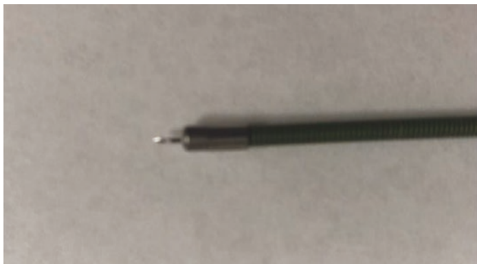
FIGURE 2.9 The distal end of the endoscopic injection catheter with the needle advanced
