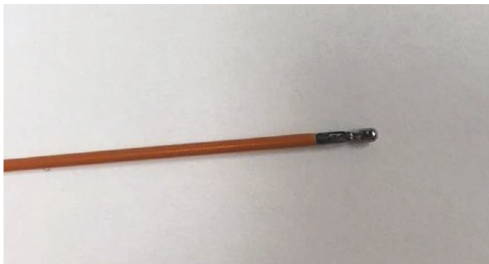
FIGURE 2.2 The distal end of an endoscopic forceps in the closed position
