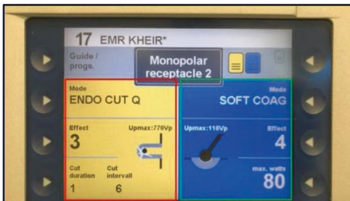
FIGURE 19.1 Example of commonly used electrocautery generator EMR settings (ERBE VIO 300D, Tübingen Germany). For resection, ENDO CUT Q mode, effect 3, cutting duration 1, cutting interval 6 (red box), and for snare-tip-soft-coagulation for controlling intra-procedural bleeding or thermal ablation of the post-EMR margin SOFT COAG mode 80 W, effect 4 (green box)
