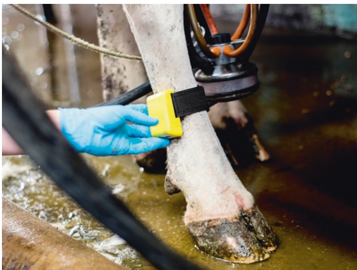
Fig. 11.3 A dairy cow wearing an IceRobotics Ice-Qube on a rear leg. Incorporating a triple-axis accelerometer, this sensor can determine when a cow is lying down, standing and, during walking, the number of steps taken. As part of the on-farm CowAlert system, it can alert when the cow is in oestrus as well as alert any changes in locomotion associated with lameness. Photograph courtesy of IceRobotics, Queensferry, Scotland
