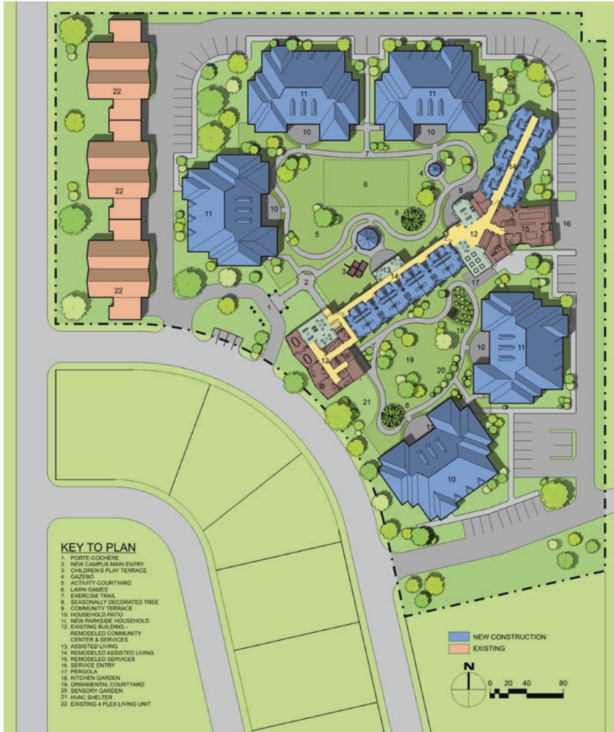
Fig. 2 The siting of the Park Homes provides passive and active secured courtyards. (Image courtesy of Jeffrey Anderzhon)
