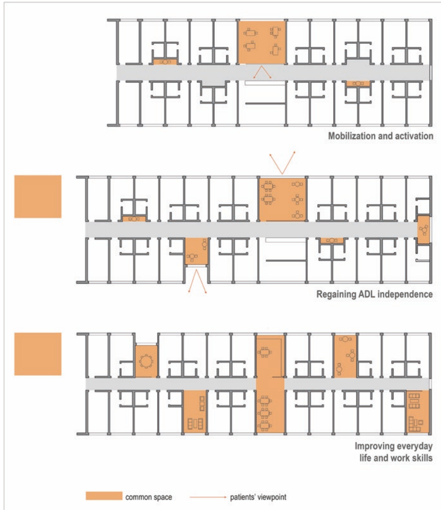
Fig. 5 Schematic floor plans of wards for patients in different rehabilitation stages: common spaces (2021). (Diagram by the author)
