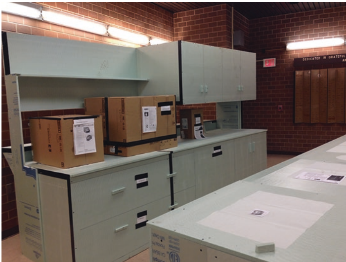
Fig. 2 Household kitchen mock-up (2015). © Perkins Eastman. Full-scale mock-ups, such as the household kitchen mock-up pictured here, were built so the design team could collect feedback from users to fine-tune the design
