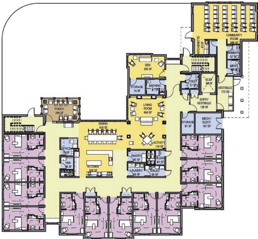
Fig. 4 Cottage ground floor plan (2015). © Perkins Eastman. The ground floor of a Jewish Senior Life cottage includes a Community Room, access to a shared outdoor garden, and a vestibule/elevator lobby that provides access to the households on the upper floors
