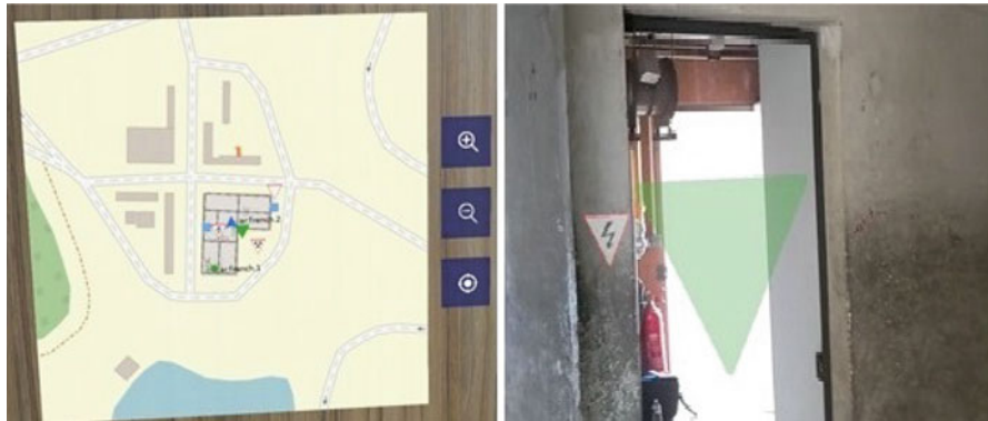
Fig. 4 The minimap (left) and POIs (right), as displayed in AR in HoloLens 2. On the minimap, the blue arrow shows the location of the user. The green dot shows another team member, while nearby POIs are also displayed
