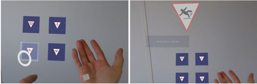
Fig. 5 POI creation from inside the HoloLens app. Left: a menu presents different types of POIs as AR buttons. Right: the POI is added and displayed in front of the user
