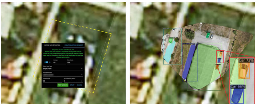
Fig. 7 Mapping and AI annotation. On the left: marking an area for mapping on the COP, setting the mission parameters, and receiving feedback regarding feasibility (in green). On the right: the results of mapping as a layer on the COP map, including AI annotations (zoomed detailed shown in lower right corner)
