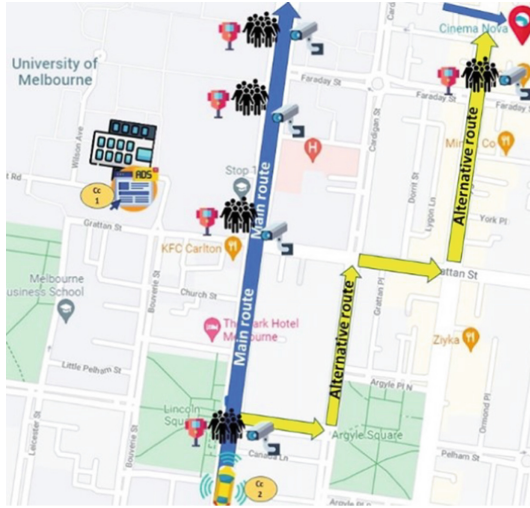
Fig. 2. Use-case- Cc 1 and Cc 2 are the marketing service agency and autonomous car respectively. Crowd icons indicate entities, and cameras to their left and right indicate video and thermal cameras. Blue and yellow arrows represent the autonomous car’s main and alternative route to reach ‘Cinema nova’ (the destination). (Color figure online)
