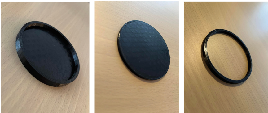
Fig. 1. The three printed models of cylindrical section pipe type, the full model and the ‘split’ model with the base and wall separated.
