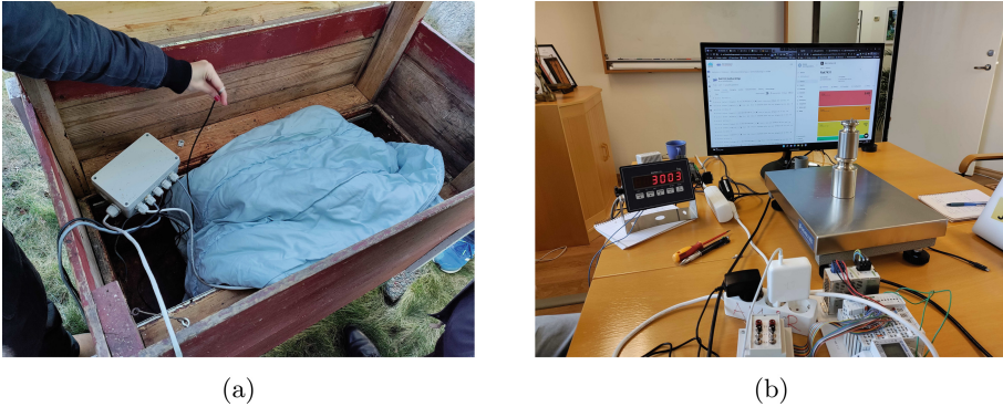
Fig. 1. (a) Traditional beehive with Raspberry Pi connected sensors; and (b) An RS-485 enabled scale sending data using LoRaWAN to The Things Network and Datacake.
