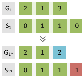
Fig. 3. Illustration of information-driven mutation operator, in which two vectors in the solution are adjusted separately.
