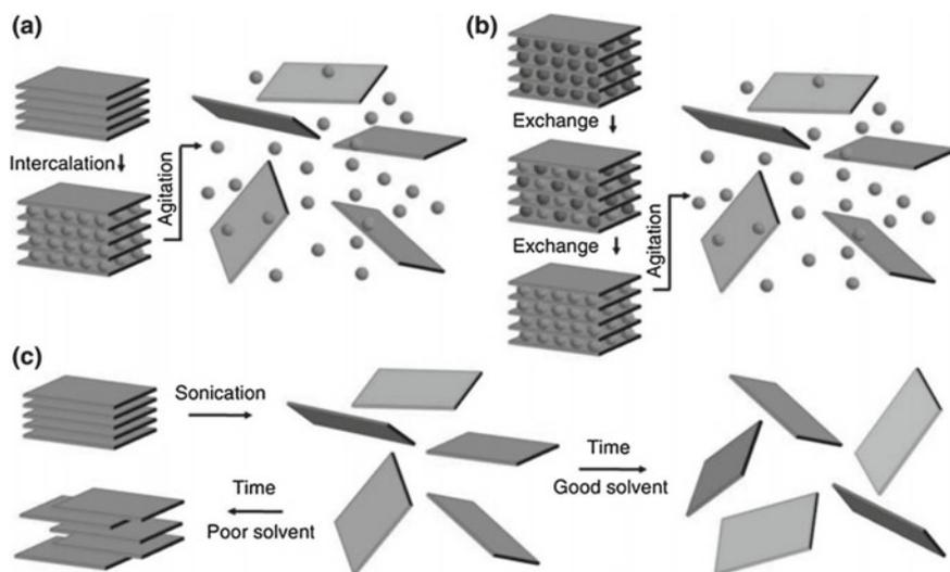
**Fig. 11.1** Schematically illustration of the liquid exfoliation process, **a** by ions intercalation, **b** by ions exchange, and **c** by sonication. The figure was reproduced with permission (Huo et al. 2015)
