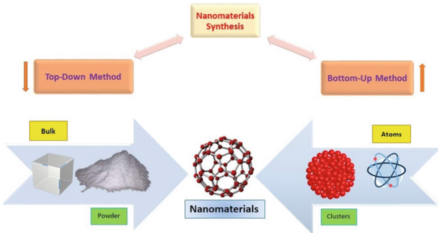
Fig. 15.2 Schematic representation of ‘top-down’ and ‘bottom-up’ methods for synthesis of nanomaterials
