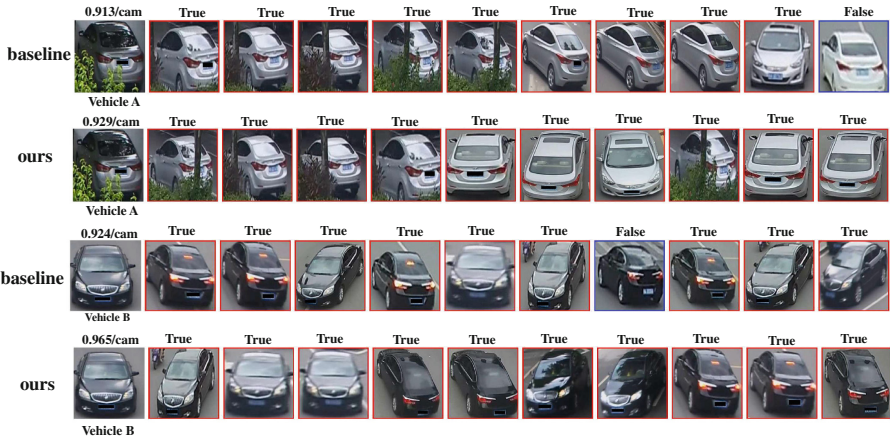
Fig. 4. Comparison of the results of our proposed method with the baseline model. The left-most column shows the test image and the right-hand side shows the top ten matches images in terms of similarity to the test image. The red box indicates a correct match and the blue box indicates an incorrect match. The indicators at the top of the Vehicle A and Vehicle B represent the mAP and cam ID respectively. (Color figure online)
