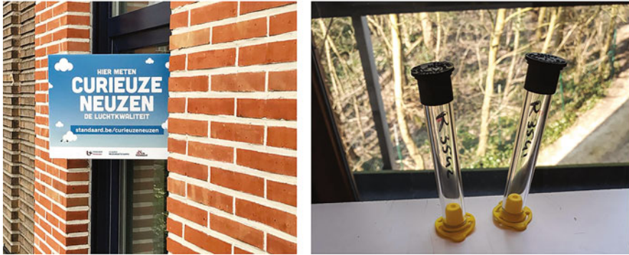
Fig. 20.3 A measurement device on a street-facing window: a window sign (on the left) and two sampling tubes that are attached on the inside (on the right) (Curieuzeneuzen, 2021)
