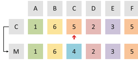
Fig. 3. Illustration of mutation operator in GA.
