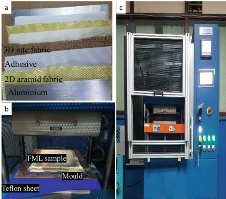
Fig. 7 FMLs fabrication process a stacking sequence of constituent material b constituents placed in the machine for the fabrication c compression hot press [46]
