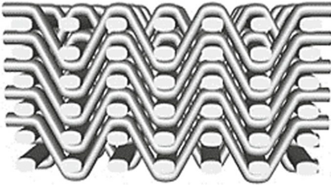
Fig. 5 Orthogonal layer to layer multilayer interlock structure
