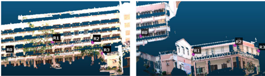
Fig. 7 Scenario 2—CPs are distributed at the bottom PC1 (left) and PC2 (right)
