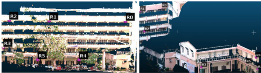
Fig. 10 Scenario 5—CPs are evenly distributed on both PC1 (left) and PC2 (right)
