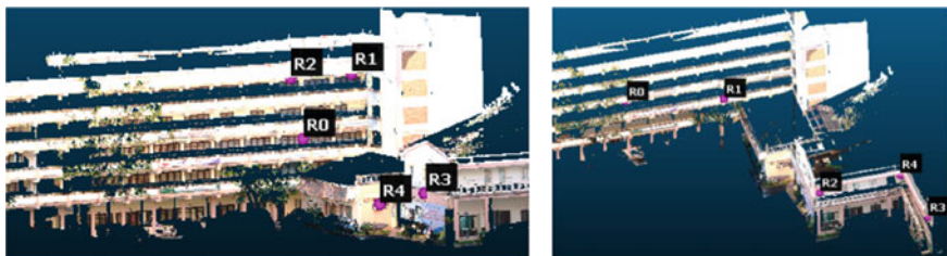
Fig. 6 Registered PC based on five tie points (left) and georeferenced PC based on five CPs (right) (Scenario 1)
