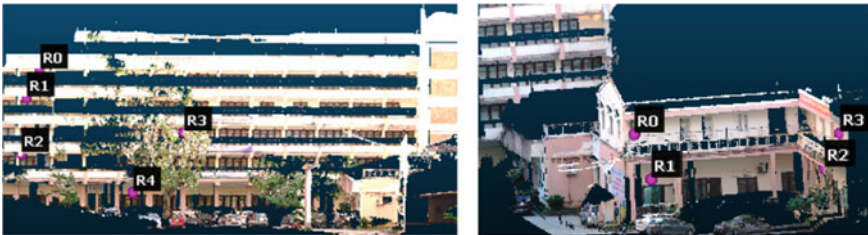
Fig. 8 Scenario 3—CPs are distributed on one side of PC1 (left) and PC2 (right)
