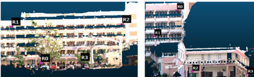
Fig. 9 Scenario 4—CPs are evenly distributed on both PC1 (left) and PC2 (right)
