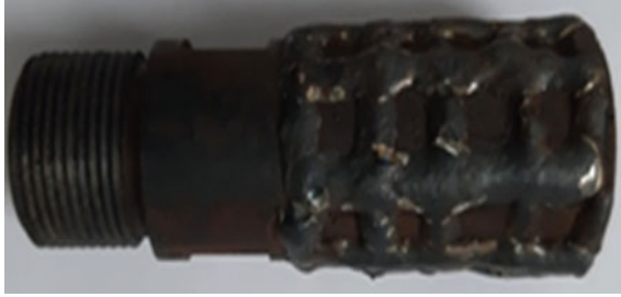
Fig. 2 A sample with surfacing on the working surface of the beaters in the form of a grid
