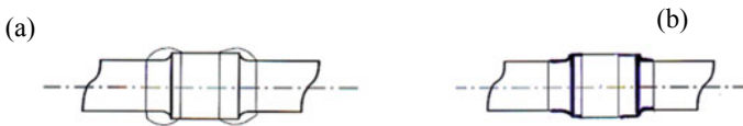
Fig. 3 Steel samples: with an anticorrosive coating (a), with a strengthened surface (b)
